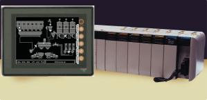
PANEL mounting) allows installation in dusty environments such as concrete batching plants.
